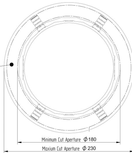
Step 2 - Install the fitting by bending up the springs 90 degrees then inserting them into the retro fit bezel aperture. Then releasing the product so that it pulls up flush to the retro fit bezel front surface. Ensure that the gasket on the product seal all the way around the aperture.
