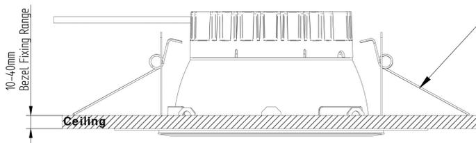
Step 6 - Fold back the springs on the retro fit bezel and place them through the ceiling void and release so that the bezel is held up against the ceiling
