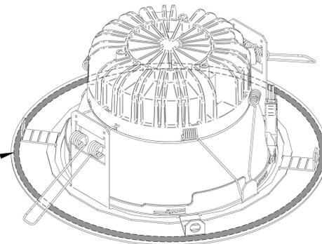
Step 4 - Apply mastic around the circumference of the bezel in one continuous loop to make a seal to the ceiling
