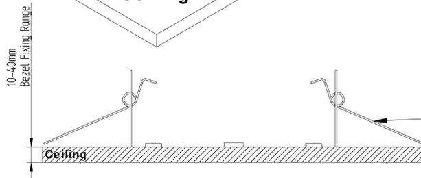
Step 4 - Wire up the driver from the product through the aperture, then install the fitting by bending up the springs and instering them into the void at 90 degrees from the retro fit bezel springs and releasing the product so that it pulls up to the ceiling.
