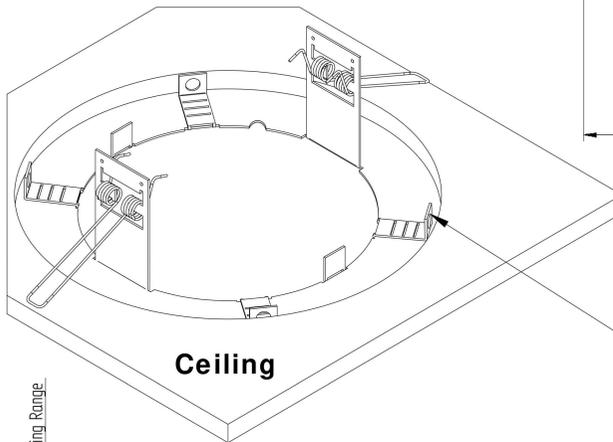
Step 2 - Fold 4 tabs as shown to centre the bezel in the hole there are a number of different easy folds for different diameters select bend closest to your hole size
