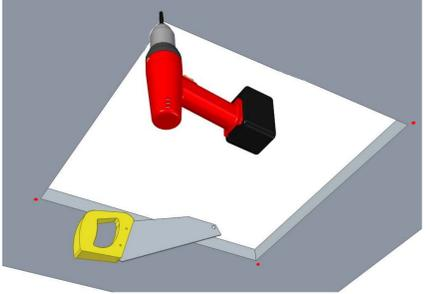
**Step 2** - Remove the ceiling bezel and 4 screws. Drill the 16 marked and 4 screw holes with a 10mm drill bit. Then cut the aperture for the fitting using the marked out lines. Ensure that the holes are drilled vertically as they need to align with the ceiling bracket cagenuts. (Cover kit will only work with 40mm Maximum Ceiling Thickness)
