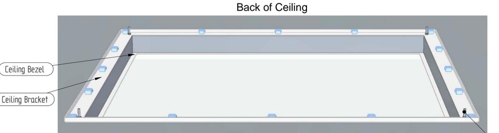
**Step 3** - Place the ceiling bracket into void and place it around the cut aperture. Then nut and bolt the ceiling bezel with dimples facing in the holes, these can be finger tight.
