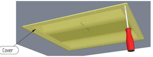
**Step 5** - Remove film from both side of cover. Make sure the counterbores for the screws are facing down. Then Screw the cover to the ceiling bracket with the 16 anti-tamper screws supplied. Engage the screws first by hand ensuring the caged nuts are not dislodged. Ensuring that screws are sufficiently torqued to 2Nm. (Security Allen key or Bit required, sold seperatly HAL-KEY3 or a 3mm security hex key)
