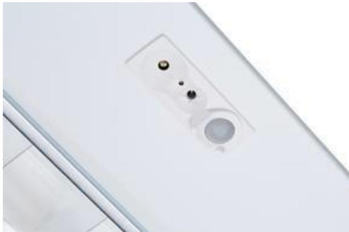
Each Sensor Node is fitted with a motion sensor, ambient light sensor, infrared transmitter and infrared receiver that allows each Sensor Node to communicate wirelessly with each of its closest neighbors.
