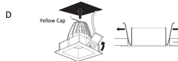
**\*IMPORTANT :- To avoid damage to soft ceiling types care must be taken when releasing the spring into the aperture.**
