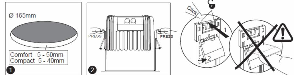
3. Feed the driver unit followed by the luminaire unit into the ceiling aperture until it is straight and the spring levers are beyond the ceiling (diagrams 3 – 6).
