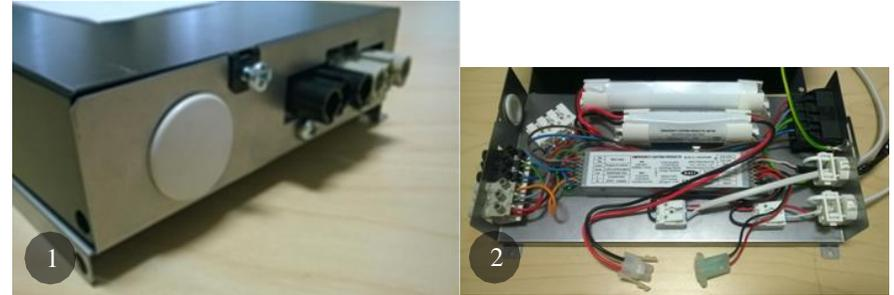
When using the COMEPS version of the emergency luminaire with a DALI driver, the emergency luminaire is supplied suitable for a combination of DALI broadcast dimming and DALI addressable emergency which require two separate DALI pairs (the dimming pair via the 6 way plug and emergency coms hard wired to the block inside the emergency box).
