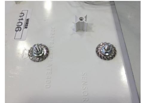
Please ensure that this is fully secured with the provided flange nuts and washers on the inside of the product before fully suspending (as illustrated above).
