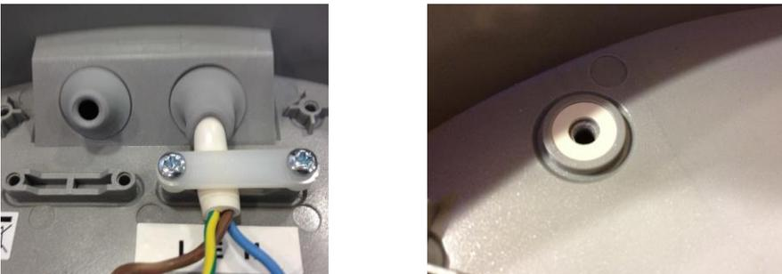
Partially fit the grub screw into the casting (as this will aid the assembly of the product), once this is done use the protruding screw and align to the arrow label on the inside of the back plate moulding, offer the casting up to the back plate and then turn anti clockwise until it locks into position;
