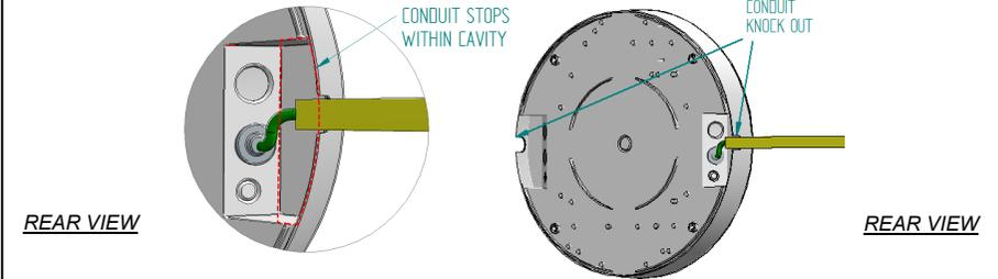
**If through wiring with conduit remove both 'Conduit Knock-Outs'.**
