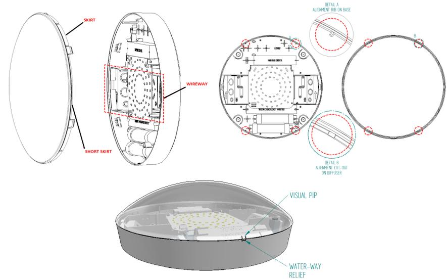
**NB Visual pips on the diffuser must align with the water-way relief cut out on the base. When the product is orientated correctly this will be at the bottom.**
