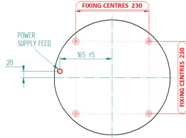
**To surface mount the product drill through the four illustrated holes on the back plate.**
