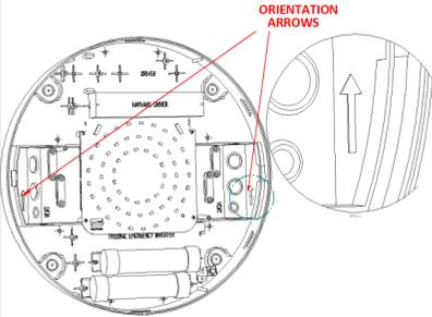
**Ensure the Arrows in the base moulding are pointing upwards**
