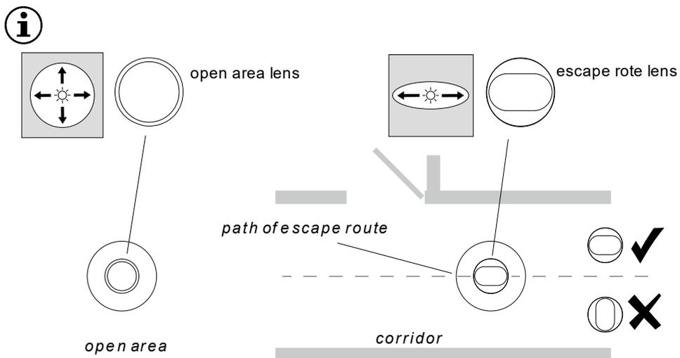
For best photometric performance ensure that the long axis of the escape route lens is in line (parallel) with the path of the escape route as shown above.
