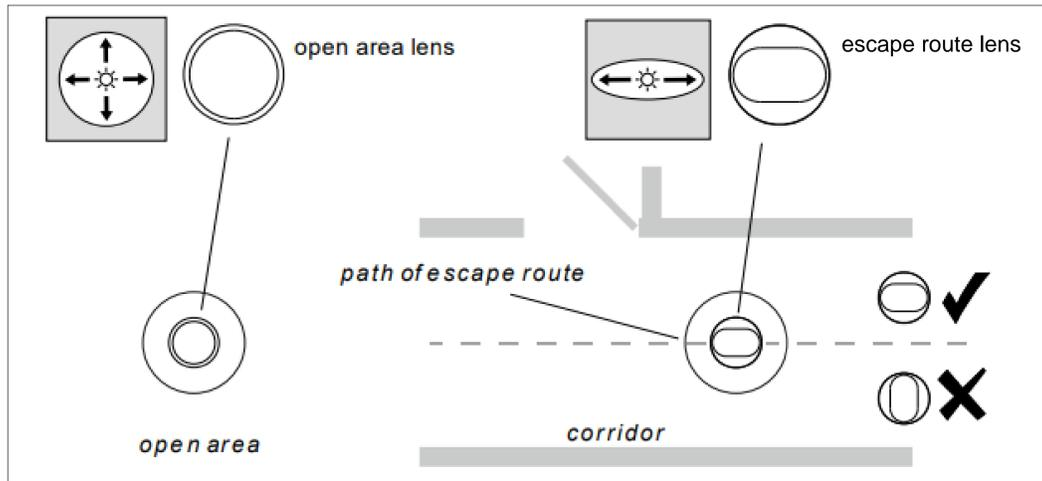
For best photometric performance ensure that the long axis of the escape route lens is in line (parallel) with the path of the escape route as shown above.
